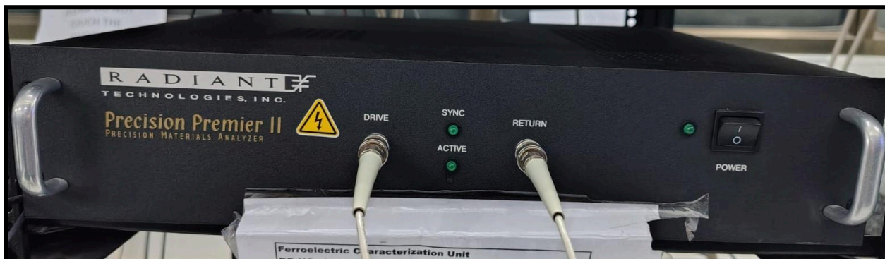
Radiant Ferroelectric Tester
